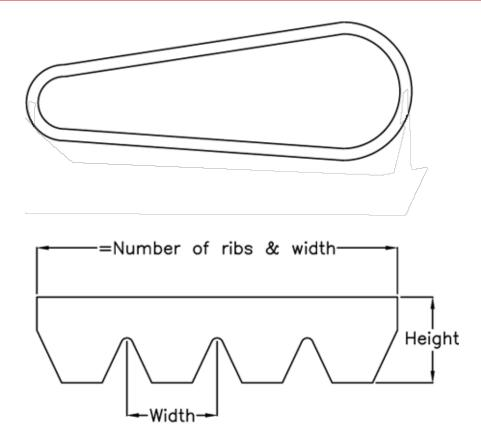
$\begin{array}{ll} \text{Datum Llength} = 1136 \\ \text{Height} &= 3.5 \\ \text{Number of ribs} = 16 \\ \text{Pitch} &= 2.34 \\ \end{array}$
